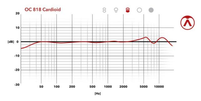
The OC818 has a frequency response similar to the famous brass CK12 capsules which is fully preserved by the open acoustic design of the microphone grill. In cardioid mode, this results in a slight boost in the upper mids starting at 3kHz to make the signal cut through even in crowded mixes.
